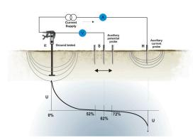
an instrument connected to test stakes positioned in the soil at measured distances from the instrument in which it injects a current into the soil and takes a measurement with the results being the resistance of the soil.
